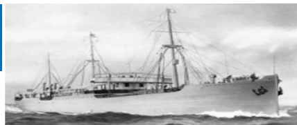
World first diesel engine ship : M/S Selandia
